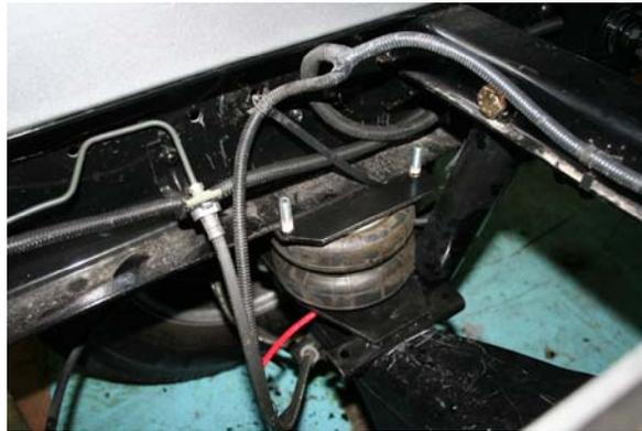
Attach the upper bracket to the reinforced frame (by taking guard than the beams and the hose connections pass in the frames)
