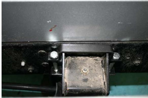
Attach the lower bracket to the frame using the bracket strap and nuts and bolts supplied as shown.
