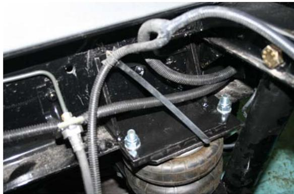
Attach the external support of the upper bracket to the chassis using the nuts and bolts supplied as shown.
