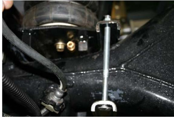
Cut a generous length of air tubing to reach from the inflation valve to the top of the nearest airspring, following the line of the inner wheel arch and across to the top of the airspring, with sufficient slack to allow suspension movement. Insert one end of this tube into the air fitting in the airspring.
