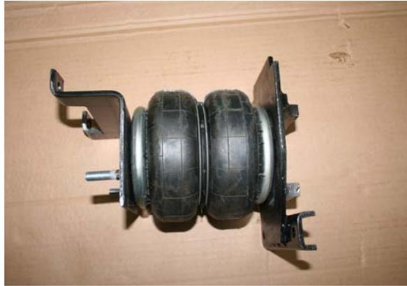
Place the assembled brackets and air springs between the axle and the chassis as shown.
