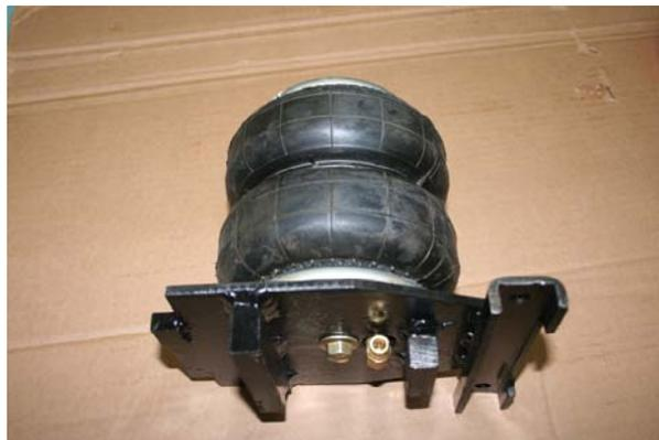
Attach the upper bracket to the airspring with the bolts supplied.
