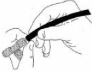
1. To cut the tubing correctly an appropriate cutter must be used (not a scissors)
