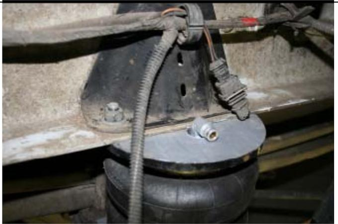
Make sure that the lower bracket is in the correct position with the axle sitting into the cut-outs in the base of the bracket and that the lip at the end of the bracket is sitting in between the leaf spring u-bolts as in the photo.
