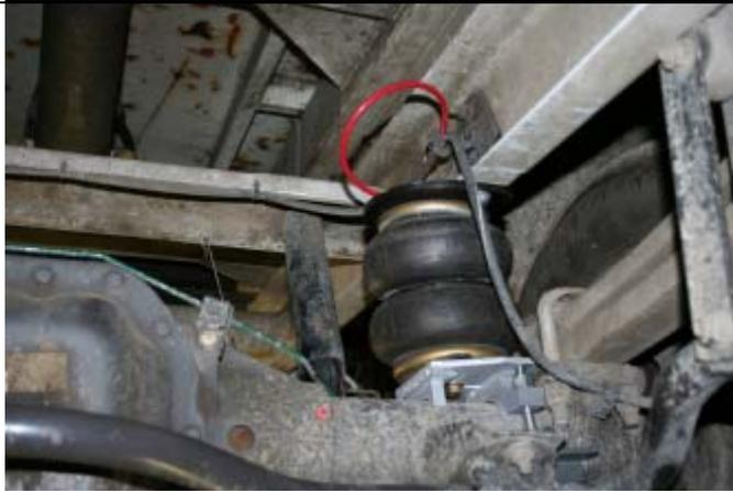
Choose whether you want separate inflation valves for each side or one valve common to both sides using the T shaped connector.
