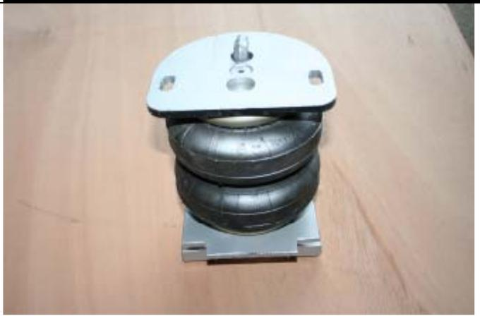
Place the air spring assembly between the chassis and the rear axle with the elbow fitting facing inboard and fix the upper bracket in place of the original bump stop using the original fasteners.
