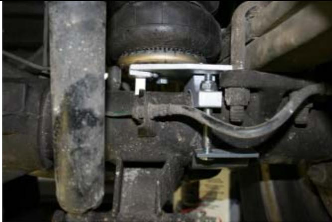
Check that the air spring assembly will not interfere with any other part of the vehicle during normal use.
