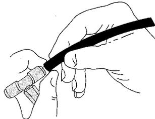
1. Cut the air tube cleanly at right angles using a special cutter or similar (not scissors). It is important to cut squarely to avoid leaks.
