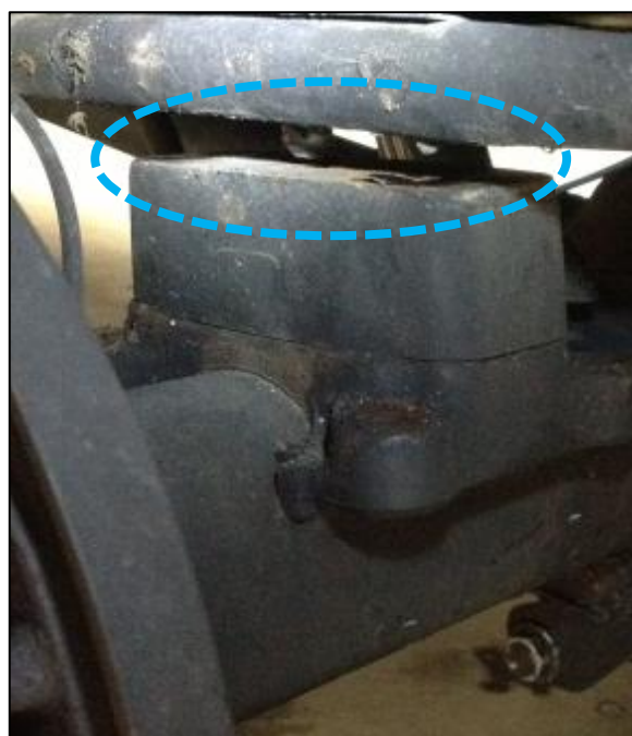
Original position of extended leaf spring spacer
