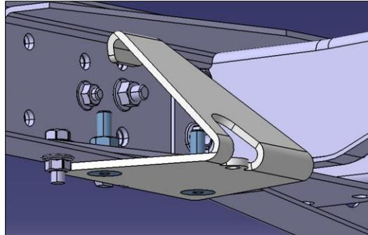
For vehicles with taller frame, fit chassis extension piece using M8 x 20 Hex Head Bolt.
