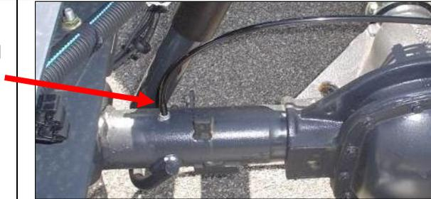
Replace with the new replacement “**De-Breather Tube**” that is supplied with the kit.
