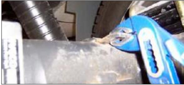
Unscrew the “**De-Breather Tube**” on the left hand side of the axle.
