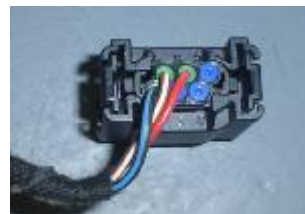
Left Height Sensor Connection
