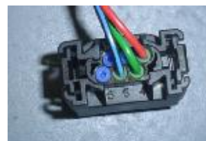
Right Height Sensor Connection
