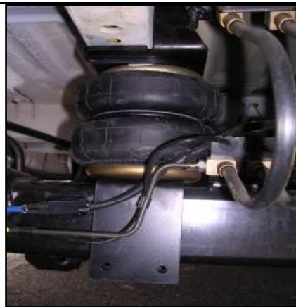
Attach the Lower Brackets to the axle using the M8x1.25-100 bolts and the M8 nuts, *do not tighten these screws yet.*
