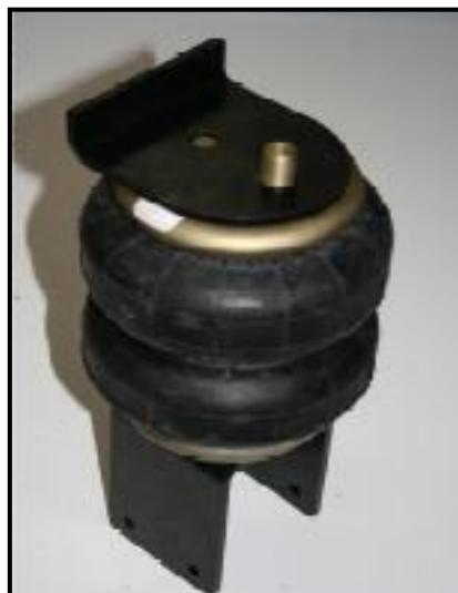
**↓ Step 4: Lower Bracket/Air Spring assembly to axle**
