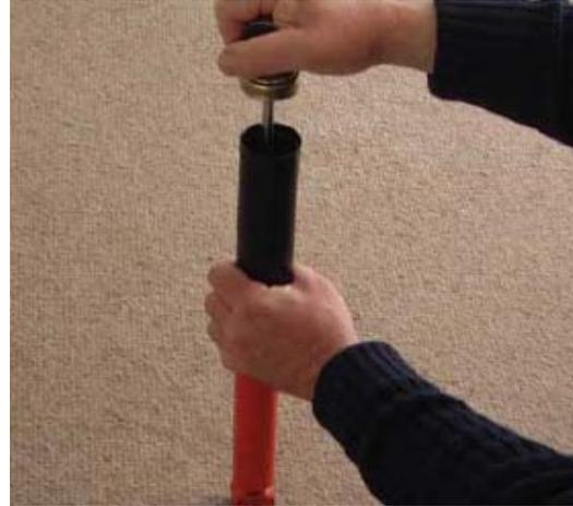
Press the button while rotating the top anticlockwise to its fullest extent. Replace the shroud.
