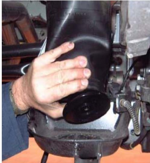
Pass M10 x 25 socket headed bolts through the M10 spring washers, and the bottom airspring plates.
