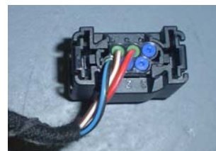
Left Height Sensor Connection
