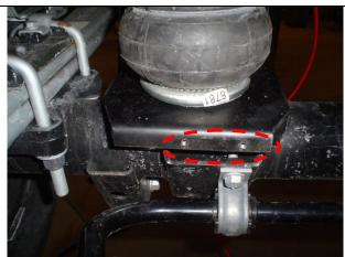
Align the holes on the clamp with the M6 holes on the lower bracket. The narrow flange should be facing in line with the axle. Bolt the clamp to the lower bracket using the M6 countersunk bolts.
