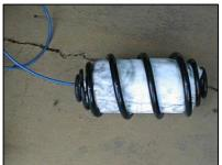
At this point it may be easier to install an air ling into the air spring before fitting the Coil Spring assembly into place. See tube lengths in Step 4.
