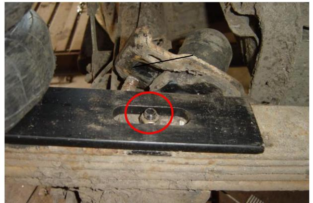
Place end of top bracket over bumper contact pad.
